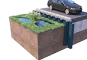
Cut-off walls used to protect places with variable or raised groundwater level
